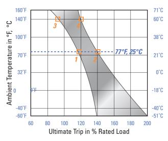
Performance characteristics are based on room temperature (77°F, 25°C). Consult Derating curve for ambient temperatures significantly higher or lower than standard room temperature.
