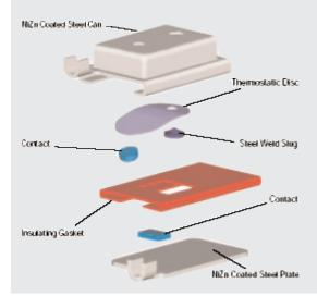
The Klixon® 7AM Thermal Protector is the market leader, backed by proven innovations in protection technology. The 7AM is a thermally operated snapaction device which delivers the maximum protection in the smallest package at an affordable price.
